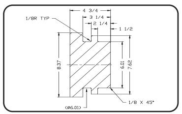
P120/120HD Bearing Spacer/Press Plate Figure 2-1
