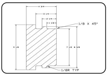
P125/P125HD Bearing Spacer/Press Plate Figure 2-1
